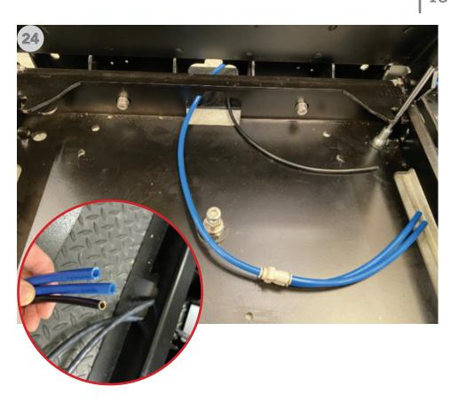
19. From the solenoid block, route, the right air supply for the shutter (black) and air supply for the air knives (blue) through the centre section into the right sensor housing, through the hole.
