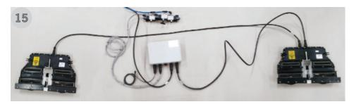
16. Route the main air supply to the solenoid block. This supply should be filtered and regulated 8-10bar.
