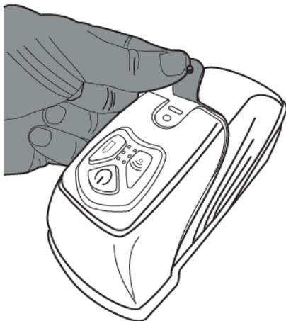
2. Plug the USB C cable into the recharging port on the lid of the scanner.
