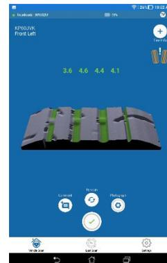
11. If scan was correct press the **[Next]** wheel button or a short press on the **Power** button, any of these action takes you to the next tyre.
