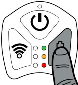
2. The battery status is then displayed on the LEDs directly to the left of the battery status button.
